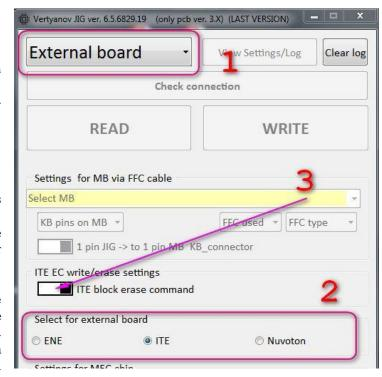
14. Work with the EC company Explore EPF035 (iROG), EPF036 / 021/011. To work with the EC of Explore, you need a pairing module - a EPF whistle. It is inserted into the side connector of the programmer.
