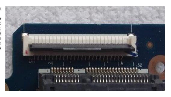
The next common mistake is since on some (not flip) connectors the contacts can be located from the top and you need to insert a loop correctly in such connector.
