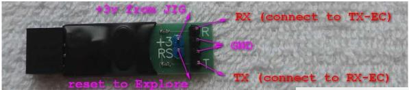
If you have a board as in the picture on the right, you need to install smd elements and you can use it to work with EC outside MB. (two R by  $10\,\mathrm{kom}$ , several C per  $100\,\mathrm{n}$ , a quartz oscillator at a frequency of  $24\,\mathrm{MHZ}$ ).
